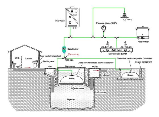
With 10 m3 family size Puxin biogas plant as per the above drawing, enough biogas can be provided to 2 families of 4 persons each for cooking and lighting.
