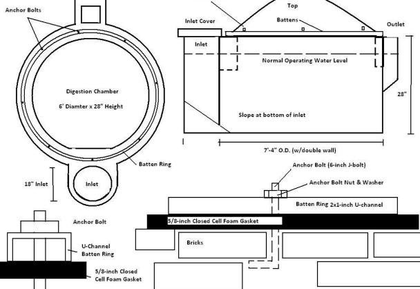
2 cu.m. Inflatable top plug-flow biogas digester
