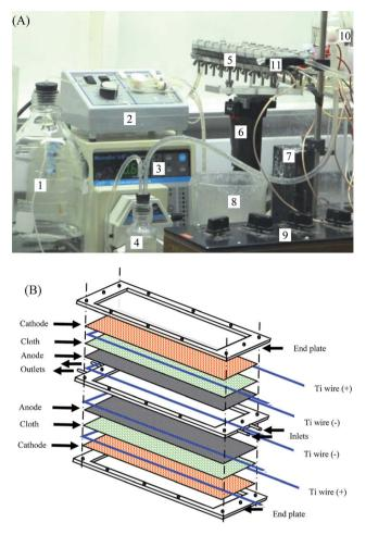
**Fig. 1** (A) A photo of the experimental setup testing the large MFC. (1) Feed bottle, (2) feed pump, (3) recirculation pump (optional), (4) recirculation bottle, (5) larger reactor, (6) tilt angle adjusting device for the reactor, (7) outlet level control device, (8) effluent reservoir, (9) precision resistor box, (10) gas sampling port, and (11) effluent outlet. (B) Schematic of the large reactor with double cloth-electrode-assemblies.
