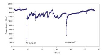
Fig. 3 Oxygen tolerance of the anodic biofilm. The performance of the CEA-MFC was not significantly affected by the direct pumping of air at a speed of 20 ml min<sup>-1</sup> and resumed quickly after the air pump was stopped.
