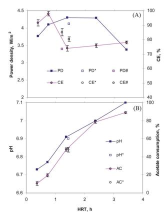
Fig. 5 Effects of hydraulic retention time on (A) power density (PD) based on CEA1 and coulombic efficiency (CE) and (B) pH and acetate consumption (AC). \*Unfilled squares and circles indicate PD and CE without the recirculation bottle. #Partially filled squares and circles indicate PD and CE without recirculation.
