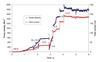
**Fig. 2** Fast start-up of a large double CEA-MFC. Power densities (solid square) are based on liquid volume and total current (open circle) is the sum of the current produced by both CEAs.
