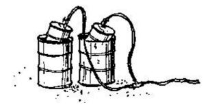
Run biogas units together
