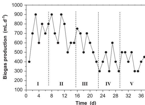
Fig. 3 – Adaptation periods of the microbial flora in the bioreactors utilizing *M. pyrifera* (algae A): (I) 3 g glucose, (II) 2.5 g glucose+0.5 g dry algae, (III) 2 g glucose+1 g dry algae, (IV) 1.5 g glucose+1.5 g dry algae, (V) 3 g dry algae.
