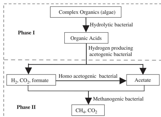
Fig. 1 – Biogas production process.
