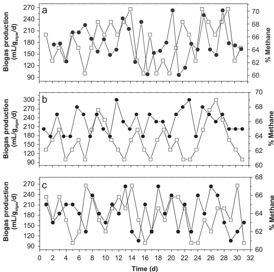
Fig. 5 – Development of the specific biogas production (□) and methane percentage (●) in an integrated system. (a) Algae A (experiment 2), (b) algae A+B (experiment 3) and algae B (experiments 4).
