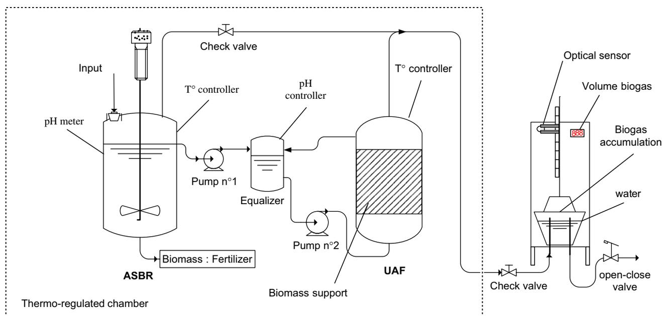
Fig. 2 – Schematic design of a two-phase anaerobic digestion system.
