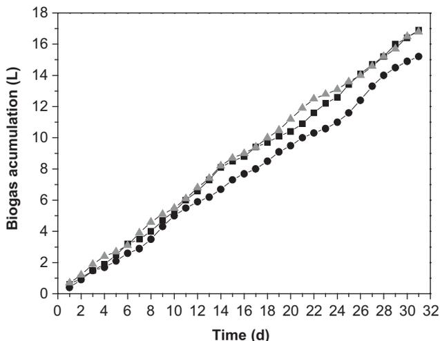
Fig. 4 – Biogas accumulation from the integrated system: experiment 2 (algae A) (■), experiment 3 (algae A+B) (●) and experiment 4 (algae B) (▲).
