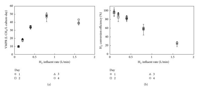
FIGURE 2: Bioreactor performance for Experiment 1. Volumetric methane production rates (a) and hydrogen conversion efficiencies (b) for bioreactor runs in which the hydrogen influent rate was varied. Data were gathered during four days. The error bars represent the observed variance between runs for each bioreactor condition within one day of experimentation.
