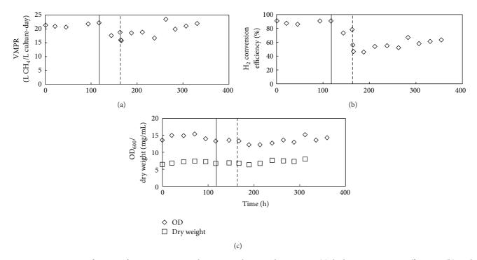
FIGURE 5: Bioreactor performance for Experiment 4. Volumetric methane production rates (a), hydrogen conversion efficiencies (b), and biomass concentrations (c) during one bioreactor run. The bioreactor was moved from the laboratory to the industrial site on hour 117 of the operating period (straight line) while untreated biogas was introduced instead of synthetic  $CO_2$  on hour 164 of the operating period (dotted line).
