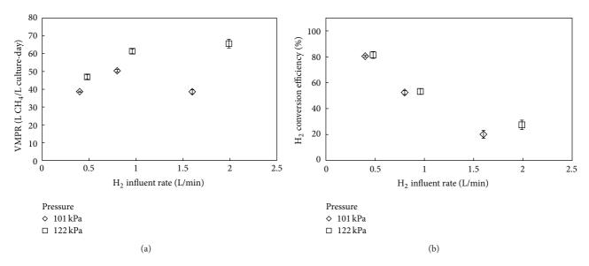
FIGURE 3: Bioreactor performance for Experiment 2. Volumetric methane production rates (a) and hydrogen conversion efficiencies (b) for bioreactor runs in which the hydrogen influent rate was varied. Data were gathered during two different headspace pressures in the bioreactor (atmospheric pressure (101 kPa) and 122 kPa). The error bars represent the observed variance between runs for each bioreactor condition.
