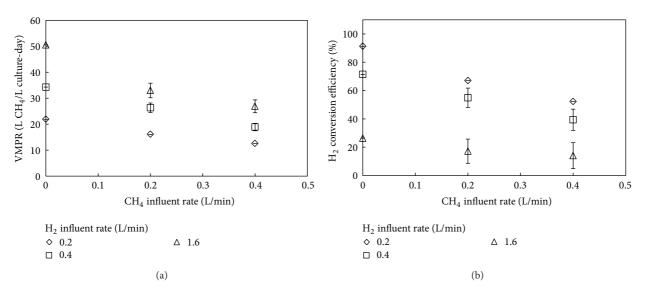
FIGURE 4: Bioreactor performance for Experiment 3. Volumetric methane production rates (a) and hydrogen conversion efficiencies (b) for bioreactor runs in which the methane influent rate was varied between 0 and 0.4 L/min. Data were gathered for three different hydrogen influent rates. The error bars represent the observed variance between runs for each bioreactor condition.
