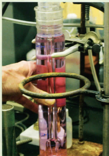
A plastic tube is part of the process for removing CO2 from the biogas.
