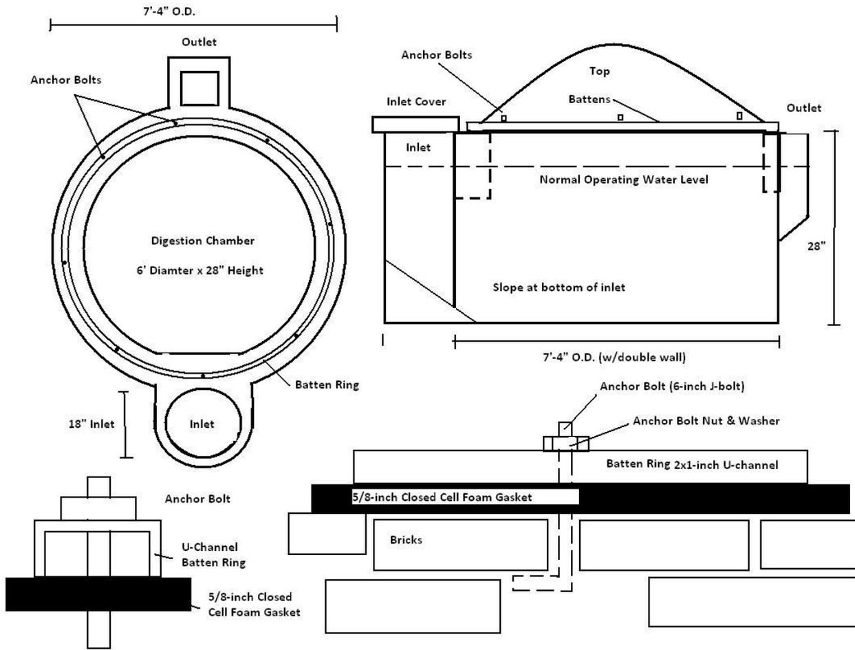
2 cu.m. Inflatable top plug-flow biogas digester
