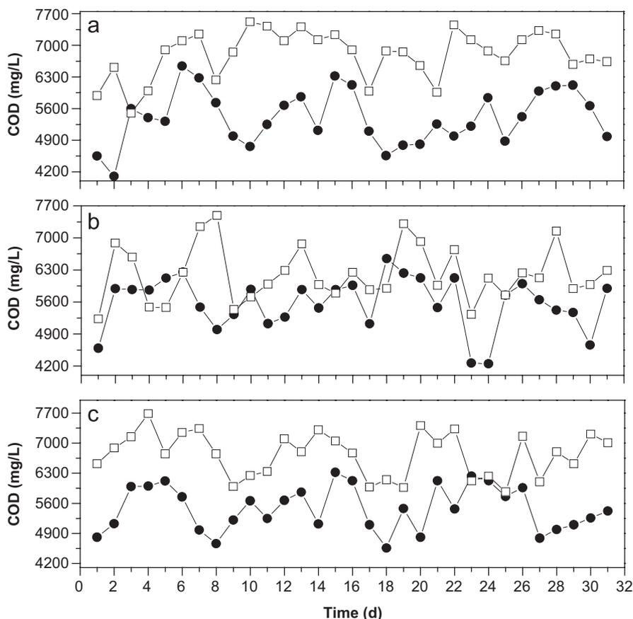
Fig. 6 – Development of chemical oxygen demand (COD) in the ASBR (□) and UAF (●). (a) Algae A (experiment 2), (b) algae A+B (experiment 3) and algae B (experiments 4).
