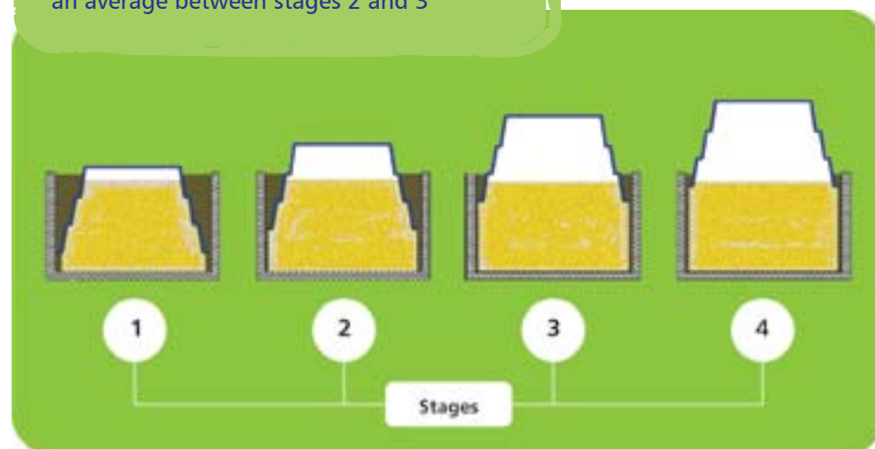
[Figure 45] Fibre Tank Elevation Stages. It is recommended that the elevations oscillate on an average between stages 2 and 3
