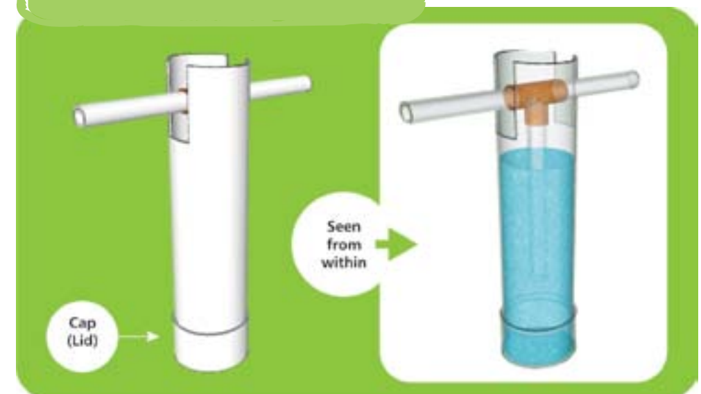
[Figure 41] Drainage Functioning System installed in the gas piping
